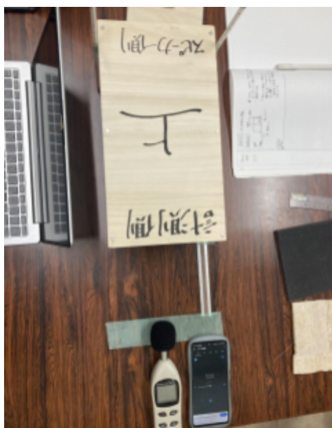
図8:へチマ吸音実験の様子③
