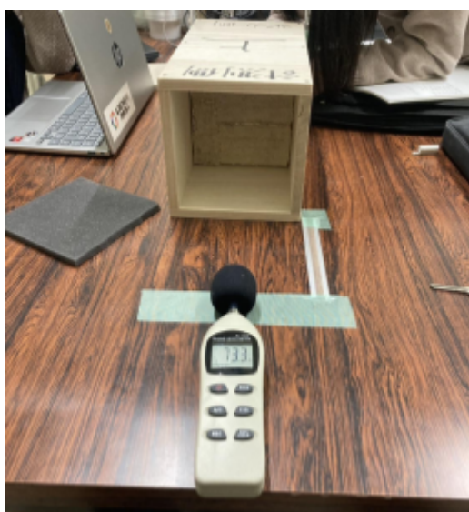
図6:へチマ吸音実験の様子①
